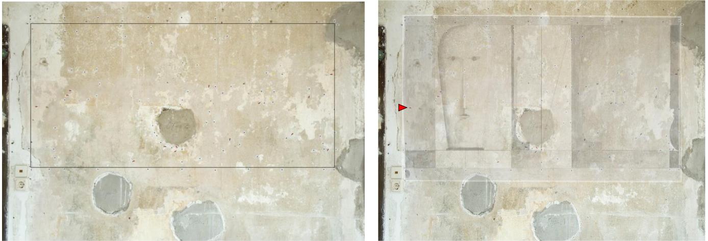
Fig. 2. The picture on the right side shows the today's status of the wall painting "Fries with heads" with sampling points. The picture on the right side shows an optical overlay with the dimensional equalized historical photograph. The red triangle depicts the sample coordinates selected as example in Fig. 3.
