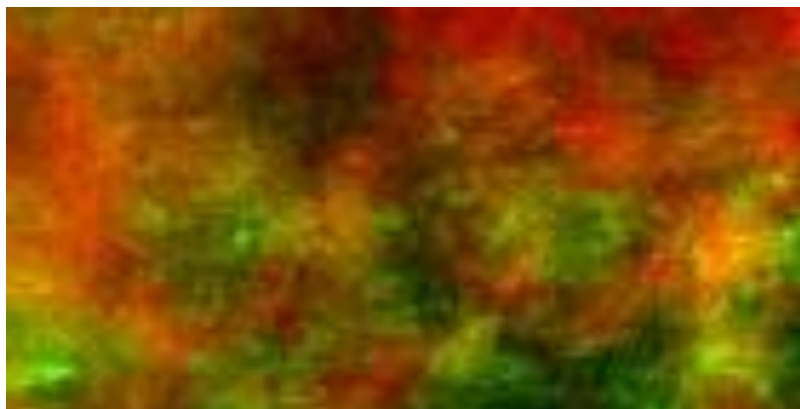
Figure 1 2D XRF map of the NiFe/Al 2 O 3 catalyst, Ni red, Fe green
