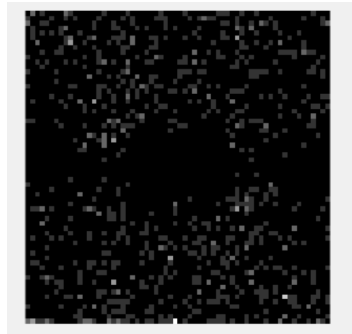
Figure 2 – Cumulative image of pairs in the energy range of 9.5 – 11.5 keV that conserve energy with a pump of 21 keV after a few hours of measurements.
