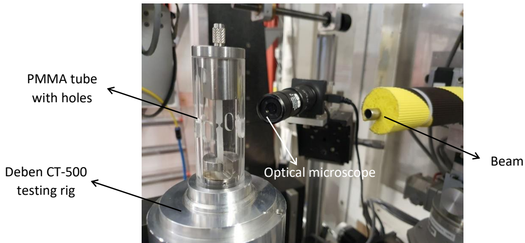
Fig. 1. Test setup at the 3DXRD station including Deben testing rig, beam and optical microscope.
