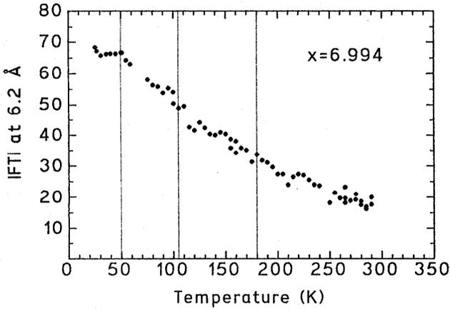
**Fig 1.** Temperature dependence of the Y-Cu<sub>2</sub>-Ba ( $6.2 \text{ \AA}$ ) MS-signal in  $\text{YBa}_2\text{Cu}_3\text{O}_{6.99}$ .
