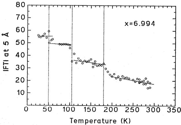
**Fig 2.** Temperature dependence of the Y-O<sub>2,3</sub>-Ba ( $5 \text{ \AA}$ ) MS-signal in  $\text{YBa}_2\text{Cu}_3\text{O}_{6.99}$ .
