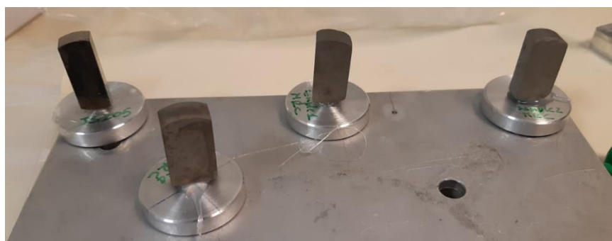
Figure 2: picture of some cut samples mounted on the sample holder before mounting on goniometer.
