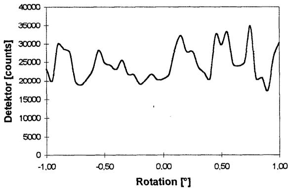
Fig. 2 Intensity of a main clathrate reflection vs. sample rotation
