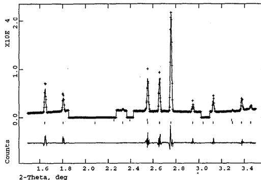
Fig.3 Rietveld profile refinement fit for the 1000 bar H<sub>2</sub>O sample
