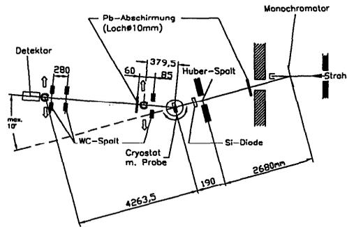
Fig. 1. Experimental set-up for the high energy powder diffraction experiment
