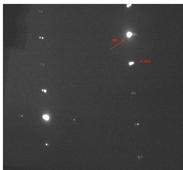
Figure 2. Reciprocal space and satellites recorded at 11K through the CCD camera, the Bragg (400) and the satellite at (0, 1/3, 0) are marked in red; b) Temperature dependence of the phonon energy on the q-points of the two satellites.
