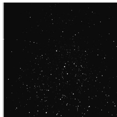
Fig. 2. Laue microdiffraction pattern of a sapphire single crystal recorded at 1200 °C. Many of the small diffraction spots spread on the diffraction image are due to the beryllium done
