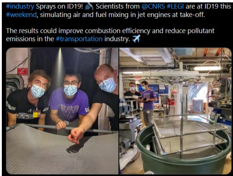
Figure 2. Screenshot of the tweet from ESRF communication service. The left picture shows the spray with O. Tolfts, N. Machicoane, and A. Rack (left to right) during set-up. The right picture highlights the spray collection system (green pool and grids) that prevents droplet recirculations and splashing. The nozzle is held by a 3-axis translation stage with an aluminium frame to allow for measurements at various locations of the spray development region by moving the atomizer with respect to the (fixed) beam. The emergency stop of the translation stage was placed outside the hutch. Air and water tubings were managed to prevent bending and pulling during translations.
