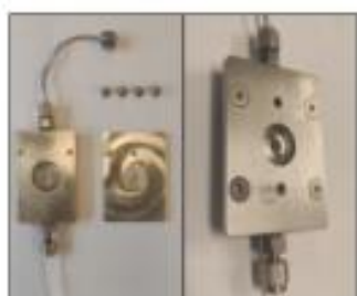
Figure 1: schematic of the in-situ setup used (left) and detail of the flow cell used for HE-XRD (right).
