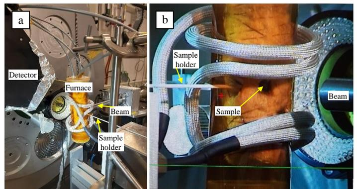
**Figure 1:** a. Experimental setup inside the hutch. b. Detail of the insertion of the sample in the furnace.
