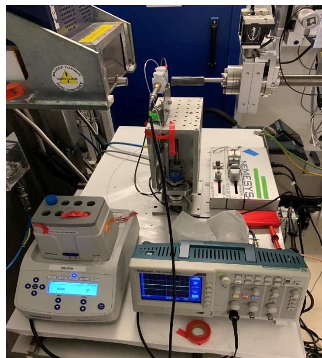
Figure 2: Flow cell for the electric field delivery device mounted in hutch.
