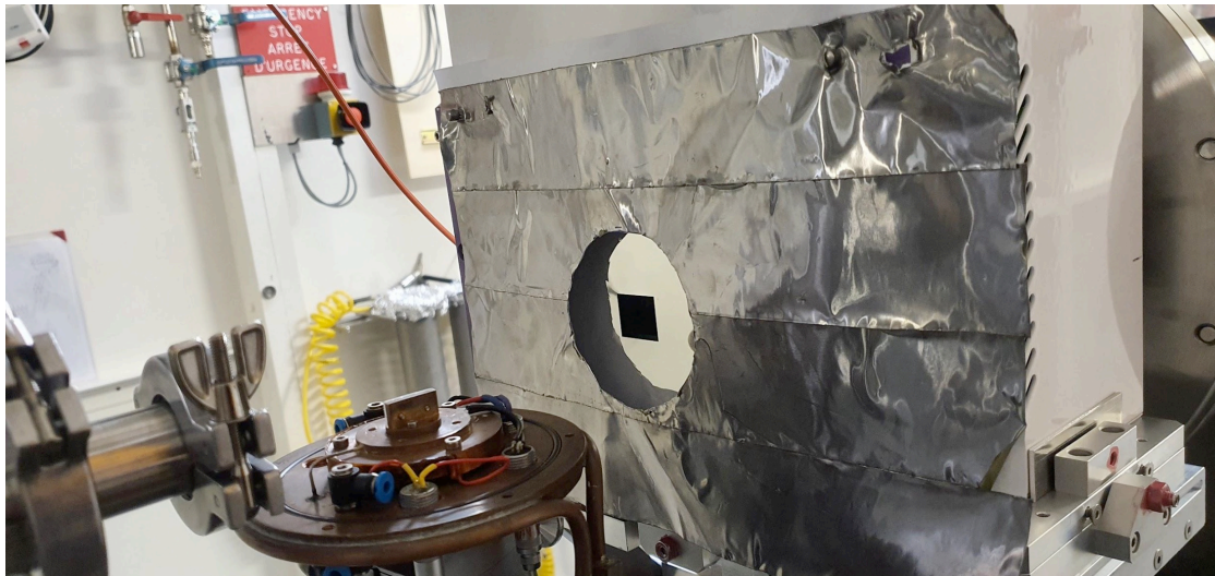
Fig. 1 Self-made mask on WAXS detector and custom-built copper sample cell.
