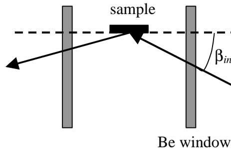
In a cylindrical sample chamber, the path length traversed by the X-rays through an absorbing medium (Be window, liquid etc.) will depend on the incoming or outgoing angles, see figure. We discuss here only the incoming beam, the exit beam is completely analogous. For incoming angle equal to zero ( $b_{in} = 0$ ), the transmission is equal to:
